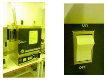
d. Check to see that the pump is on, the oil level and cleanliness(If off turn Vacuum Pump on)
