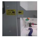
For the best safety results make sure that the arrows line up on the sash and the bench before Beginning any etch process. Always cover containers when possible to minimize the amount Of vapors. You will notice a white streamer at both ends of the sash as a visual indication of exhaust. But do not depend on this indicator alone but as a secondary indication.
