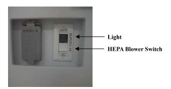
On the right side of the bench are two rocker switches. The top switch which is black is Used to turn on and off the fluorescent lamp within the bench. Which is also indicated by the word **LIGHT**. The lower switch is white and indicated with the word **HEPA**. This switch turns on and off the blower that supports the HEPA filter. This blower **RUNS 24/7 AND SHOULD NOT BE TURNED OFF EXCEPT FOR EMERGENCIES**.
