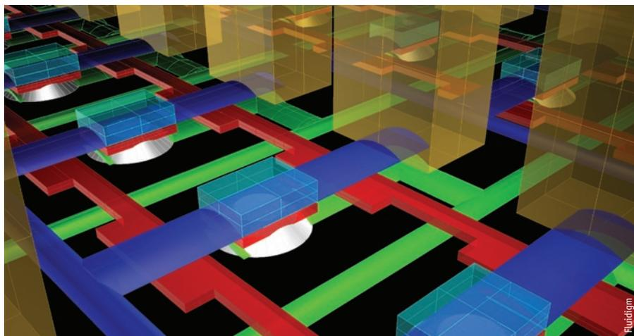
Fluidigm relies on the process of multilayer soft lithography to generate channels and valves when designing microfluidic devices.
