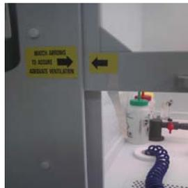
For the best safety results make sure that the arrows line up on the sash and the bench before beginning any etch process. Always cover containers when possible to minimize the amount of vapors. You will notice a white streamer at both ends of the sash as a visual indication of exhaust. But do not depend on this indicator alone but as a secondary indication.
