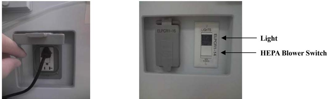
On the right side of the bench are two rocker switches. The top switch which is black is Used to turn on and off the fluorescent lamp within the bench. Which is also indicated by the word **LIGHT**. The lower switch is white and indicated with the word **HEPA**.
