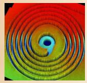
An optical profile image of an inertial microfluidic device for rapid fractionation of blood. The spiral microchannel with a central input and three perimeter outputs is formed in elastomer by soft lithography. The device takes advantage of the inertial effect of fluid around blood cells to drive them across flow streamlines into equilibrium positions, leading to fractionation of blood into red and white blood cells in minutes.
